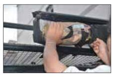
**3.** Unzip weather resistant cover and release the mechanical fasteners, allowing the fabric to be released.
