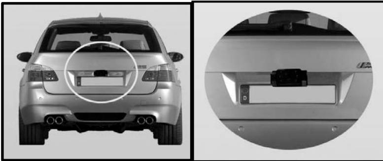
1. Remove the rear license plate, and then loosen the bolts/screws of the license plate.
