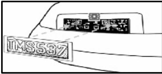
4. Choose a routing path for the camera's power cable through the vehicle's body to the reverse light circuit.
