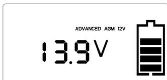
This mode is mainly suitable for charging 12V lead-acid batteries with a capacity greater than 18 Ah. It can be used to the maximum charge voltage 15V of the special AGM battery such as calcium battery; however battery manufacturers may recommend the maximum charge voltage for charging their batteries. Please check battery specifications.
