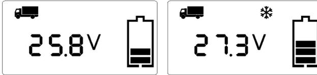
This mode is suitable for charging 24 V lead-acid batteries with a capacity less than 10 Ah.
