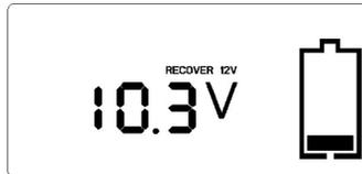
This mode is mainly suitable for charging 12 V lead-acid batteries with a capacity greater than 18 Ah. Long press 3 sec. the MODE selection button, if the measured voltage is between 2.0 V and 14 V the battery is identified as a 12V battery to activate **RECOVER 12V** mode.
