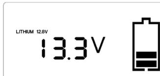
Long press 3sec. the MODE selection button, if the measured voltage is between 11.6 V and 13.8 V the battery is identified as a Lithium (12.8V 4-cells LiFePO4) to activate **LITHIUM 12.8V** mode.
