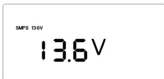
This mode is adaptor, it can be used to as a 13.6V 5.0A DC power supply, and it can be used to float charging for 12V battery also.
