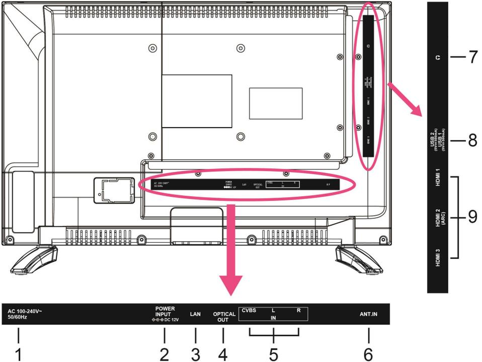
1. Power input: Connect to the mains outlet via the mains plug.
