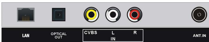
Use OPTICAL cable (not included) to connect the unit with amplifier or other audio decoding devices for digital audio signal output.
