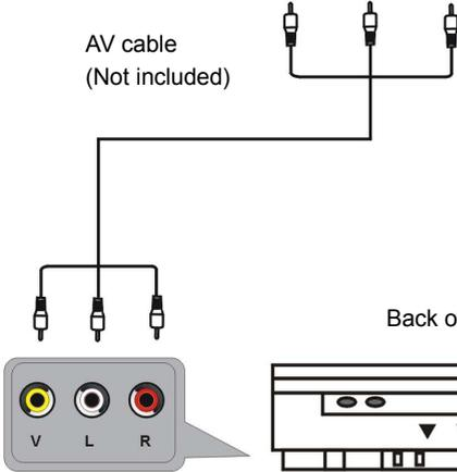
For basic connection, use the composite Audio L/R (white/red) and CVBS (yellow) cable to connect the unit with other devices.
