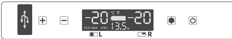
H should be set when the product is connected to car power, and M or L should be set when it is connected to a portable battery or other back-up battery. The battery protection level should be set to H if the product will keep working after turning off the car engine, or the product may drain the battery.
