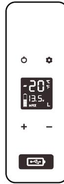
H should be set when the product is connected to car power, and M or L should be set when it is connected to a portable battery or other back-up battery. Because of the different output voltages between vehicles, the battery protection level can be set from H to M or from M to L if there is a voltage protection code F1 shown on the panel. The battery protection level should be set to H if the product will keep working after turning off the car engine, or the product may drain the battery.
