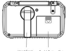
Hand Crank 3 x AA Battery Slot
